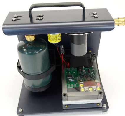
Propane Unit & Controller
