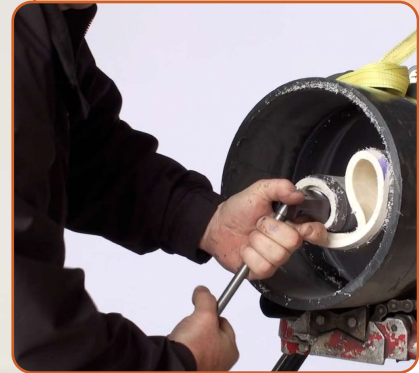
Twist and Extract and Reuse Pipe
